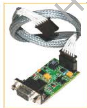
Insulated serial interface RS232, enabling the direct connection to a printer or PC. Only with optional TE550 control. Option 50214.
